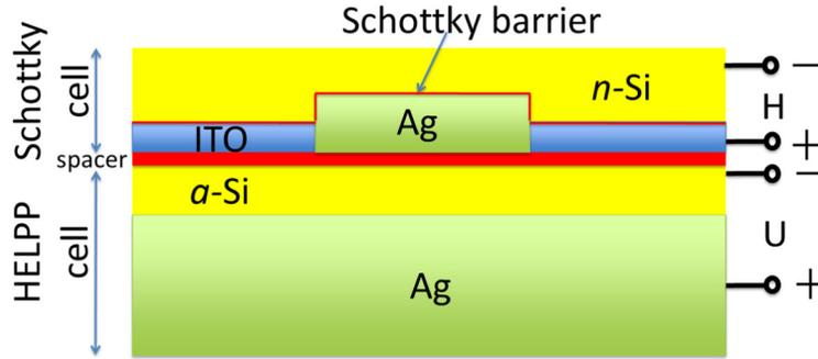
Fig. 4. Schematic of a tandem hot electron cell, with a thin plasmonic resonator-embedded Schottky junction generating voltage  $H$  (for hot) separated from an ultrathin solar cell ( $a$ -Si shown) generating voltage  $U$ .
