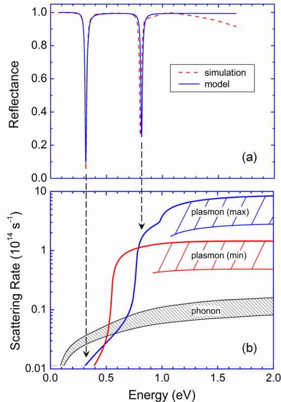
Fig. 2. (a) Reflectance of the structure shown in Fig. 1: simulations (dashed line) and model three-layer system calculations (solid line). (b) Calculated minimum (red) and maximum (blue)
