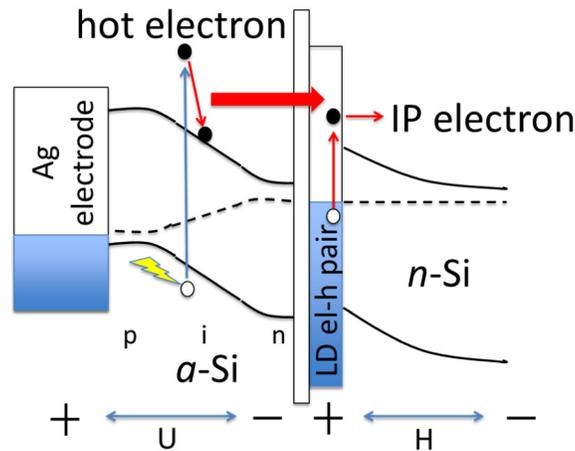
Fig. 5. Band diagram of tandem cell of Fig. 4. IP is inverse photoemission process for hot electron energy release from plasmonic resonator. LD refers to Landau damping.
