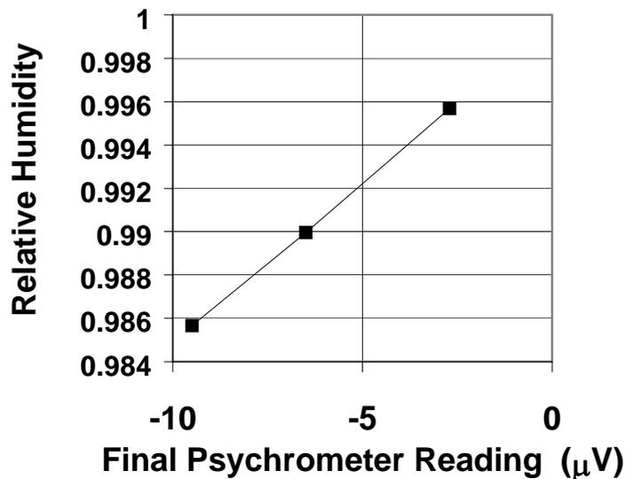
Figure III.1 - Calibration solution relative humidity versus *final psychrometer reading* ( $\mu\text{V}$ )<sub>caln</sub>.
